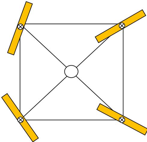
As the rotor blades turn, they push air downwards with speed  $v$ . In time  $\Delta t$ , the air that moves is within a cylinder of radius  $r$  and height  $4\rho\pi r^2 v \Delta t$  (the factor of 4 is there because there are 4 blades); its momentum changes within this time by  $\Delta p = 4\rho\pi r^2 v^2 \Delta t$ . Thus, the force exerted on air is
